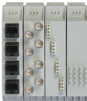
DNX BACKPLANES (RJ48, BNC, IDC, WW)
